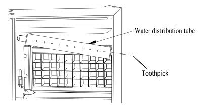
When you find the ice cubes are incompletely formed or the output is low, the water distribution tube may be blocked. Turn off the power button, gently take out the water distribution tube, locate the holes in the distribution tube and use a pointed object such as a toothpick to dredge the holes. Then put the water distribution tube back to its original position. If the tube is badly blocked, clean it as follows:
