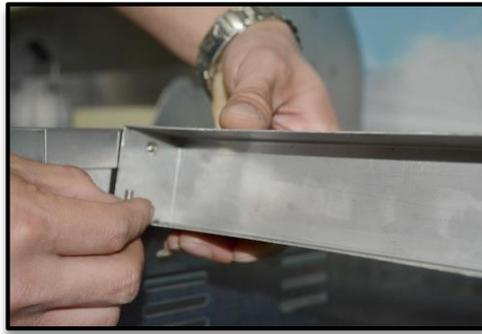
**Step 4:** Attach the Right & Left Side Shelf Brackets (Arrow pointing up) to both sides of the cart,
