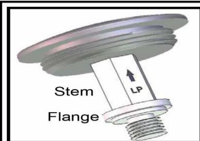
Step 4: Screw the Stem back into the Cap and then reinstall the Cap/Stem Assembly back into the Regulator.
