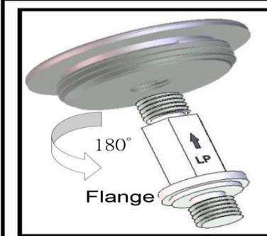
Step 3: Turn the Stem 180° so that the Flange is at The Bottom.
