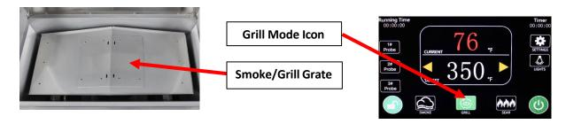
• <u>SEAR</u> Mode - (Must use the Sear Grate in this mode) - Allows you to cook directly over the flame at high temperatures to sear in the juices. To use the Sear mode, press the Sear mode icon. The grill will automatically begin the ignition process. Press the Low, Medium, or High buttons to control the sear temperatures. To exit Sear mode, press the Sear button, and the grill will go back to the last grill mode and temperature setting.
