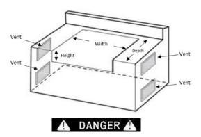
A minimum of 2 vents, but optimally 4, is required per cabinet. Each vent must be at least 20 sq. inches and have access to outside/fresh air.
