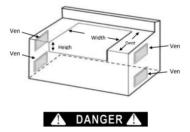
Cabinets with any gas supply or connection must have at least two vents, ideally four for optimal performance. Each vent should be a minimum of 20 square inches and provide direct access to outside or fresh air. To ensure adequate airflow and ventilation, it's advisable to install two vents on each side of the cabinet.
