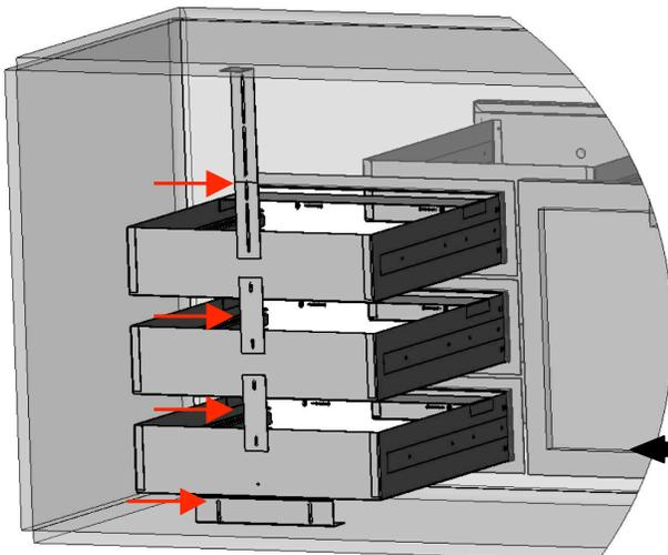
Rear view of installation details. Red arrows indicate parts that are included with the Modular Drawer Kit (Model LMD-KIT) allowing the individual drawers to be stacked 2 or 3 high.
